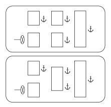
The front passenger seat with power adjustment does not have a tether anchor. The two tether anchors on the back of the second row bench seat can be used either for child safety seats at the two seating positions, or either anchor can be used for a single LATCH child seat installed at the center of the bench seat.
